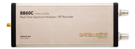
Speed link. It has 27 MHz of real-time bandwidth, tunes from 9 kHz to 6 GHz, collects 80 million samples per second, and streams data to your computer at 140 MB/sec. By adding a high-speed hard drive to your PC or laptop (250 MB/s sustained write speed), the BB60C doubles as an RF recorder, streaming up to 80 million IF samples per second, or 40 million I/Q samples to disk.
