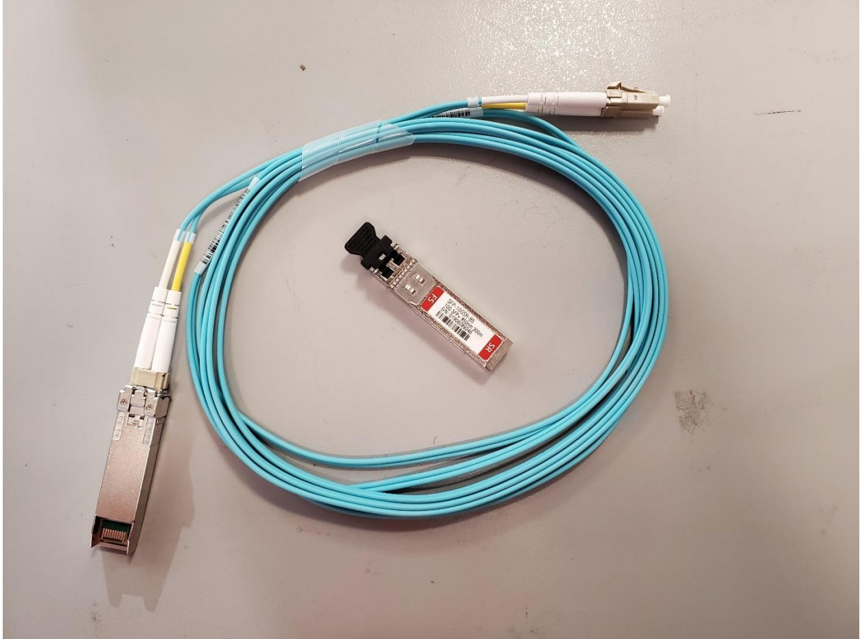
Figure 4: Multi-mode fiber cable with two SFP+ SR modules, one attached and one not.
