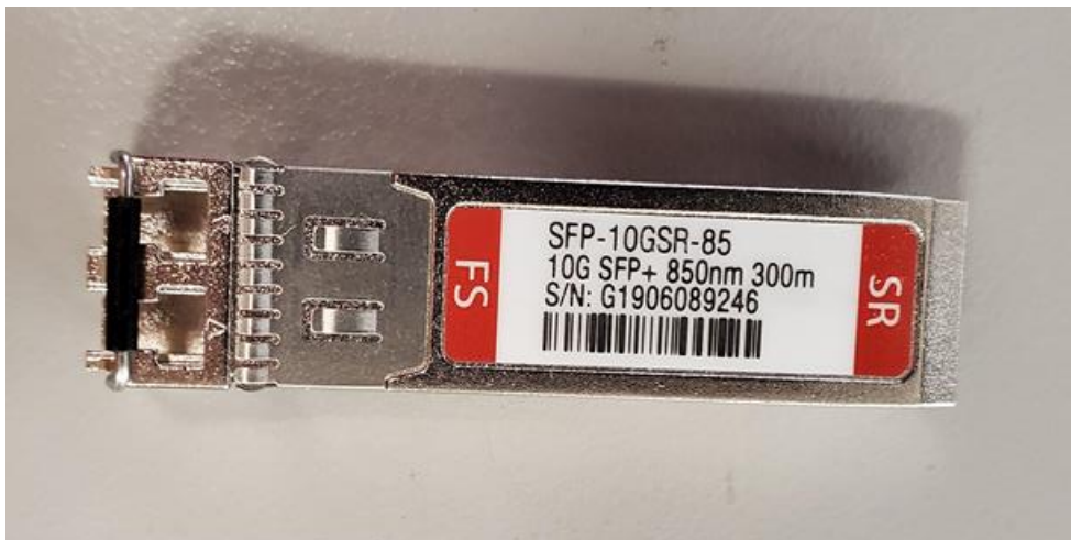
Figure 1: SFP+ 10GBASE-SR (fiber optic) module
