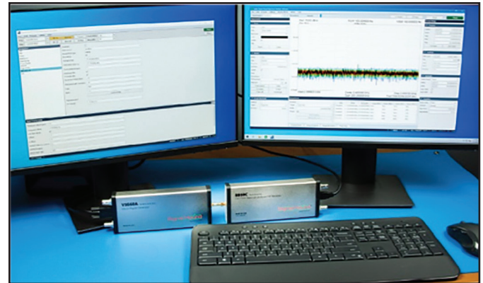
The VSG60A vector signal generator paired with our BB60C spectrum analyzer.
