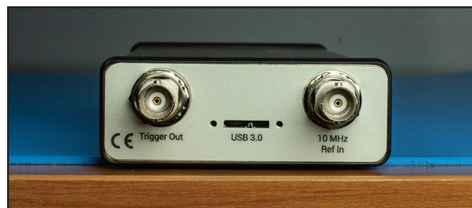
The external 10 MHz reference input of the VSG60A
